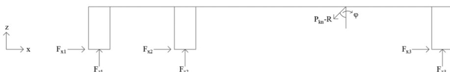
Figure 11. Longitudinal view of the structure
